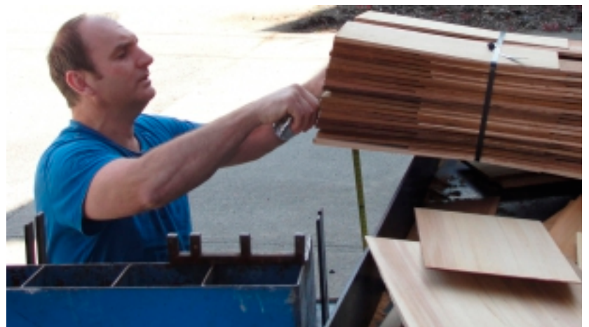
Clay Walker, CSSB Cedar Quality Auditor, checks coverage on a test bundle.
