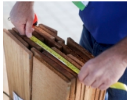
Clay Walker, CSSB Cedar Quality Auditor, measuring a bundle for coverage.
