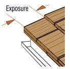
Exposure is the amount of installed product left uncovered to the weather in each course (row). Overexposing product results in loss of roof integrity and violates building code. Reduced exposure, either for aesthetics or longer life span, is a popular choice, however, ensure to calculate in the extra product needed to achieve this design.
