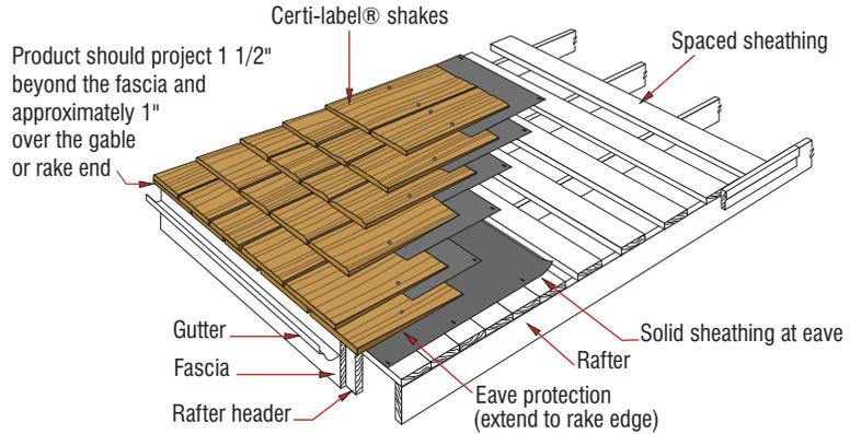
**Figure 1: Spaced Sheathing**
