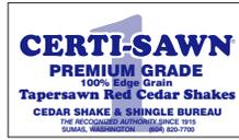
These shakes are sawn both sides. Premium and Number 1 Grades are the most common. Premium Grade is 100% edge grain, 100% clear and 100% heartwood. Number 1 Grade allows up to 20% flat grain in each bundle. Number 2 and 3 Grades are also available.
