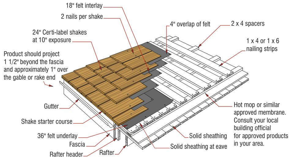
**Figure 7: Certi-label® Shake Application to Low Slope Roofs**
