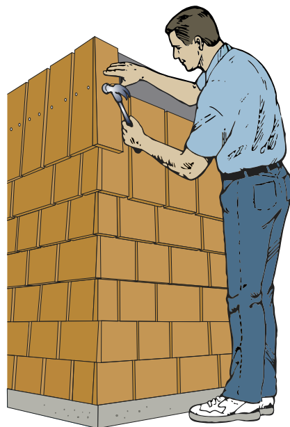
Figure 9: Fitting Laced Corner Courses
