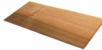
A good grade for many applications. Not less than 10" clear on 16" shingles, 11" clear on 18" shingles and 16" clear on 24" shingles. Flat grain and limited sapwood are permitted in this grade.
