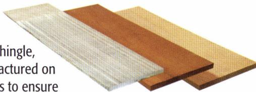
A sawn shingle, remanufactured on four sides to ensure square butts and parallel edges for superior appearance on sidewall applications. Also available with sanded or machine grooved face (Certigroove®). Predominately kiln dried. Pre-primed or pre-stained options available.
