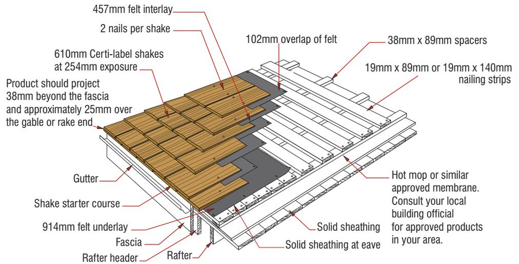
Figure 7: Certi-label Shake Application to Low Slope Roofs
